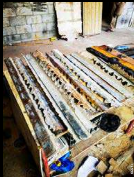
To the right: the steel combs used to smooth the finishes
